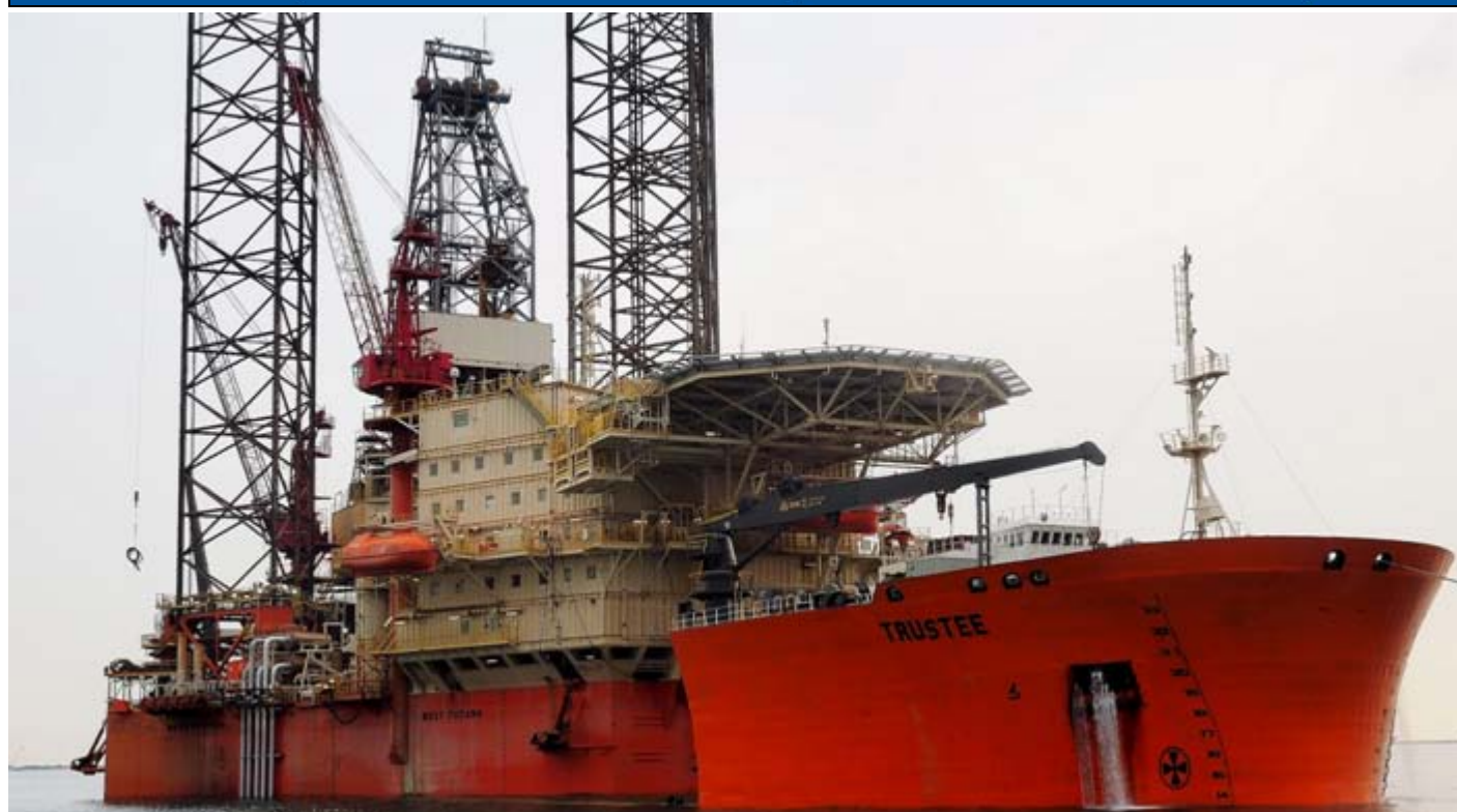
Dockwise TRUSTEE seen de-ballasting after loading of the WEST TUCANA at the West Jurong anchorage in Singapore Photo : Piet Sinke © – CLICK on the photo !
