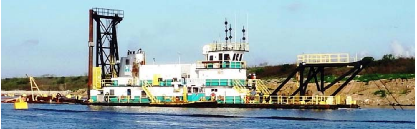
The 24-inch cutter dredger " RICHARD LAQUAY " of Orion Marine Group seen at work in Barbour's Cut, Houston Ship Channel. Photo : Alexander Pera ©
