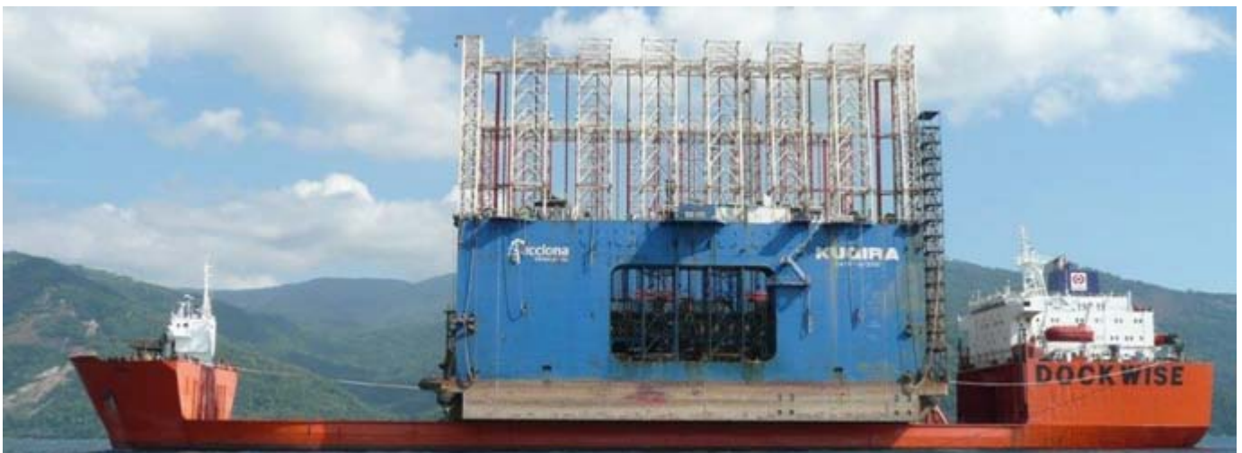
Dockwise's TEAL seen loaded with a floating dock, ready for departure from Angra dos Reis, Brazil
