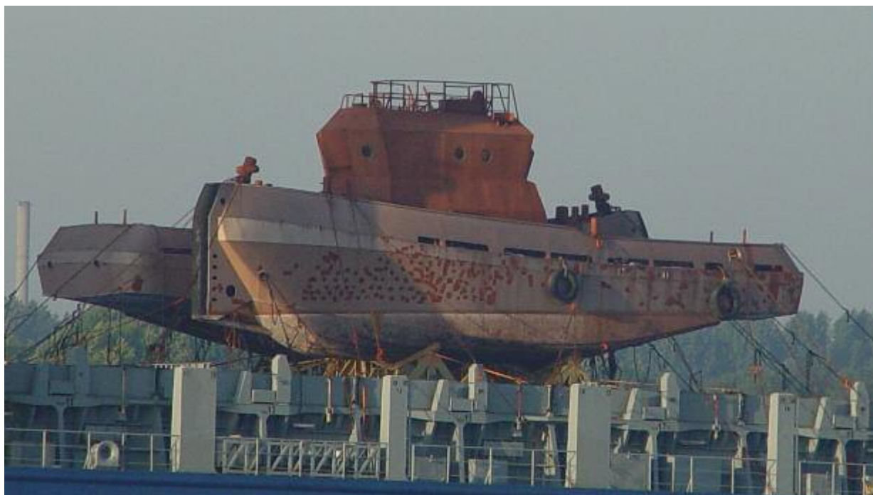
The NIRINT ATLAS arrived in Rotterdam with as deck load 2 newbuild hulls
